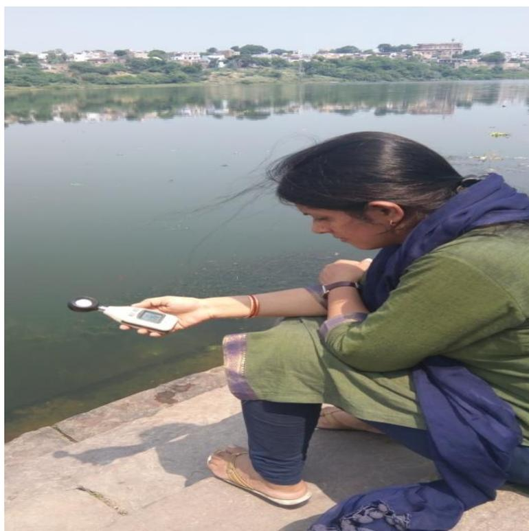
**Figure 4.2: Determination of light at the sampling station**
