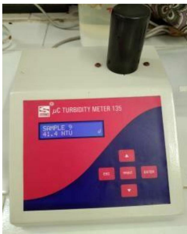
**Figure 3.4: Conductivity and turbidity meter**
