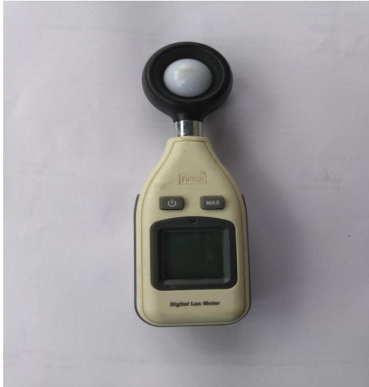
Figure 3.1: Digital Lux meter
