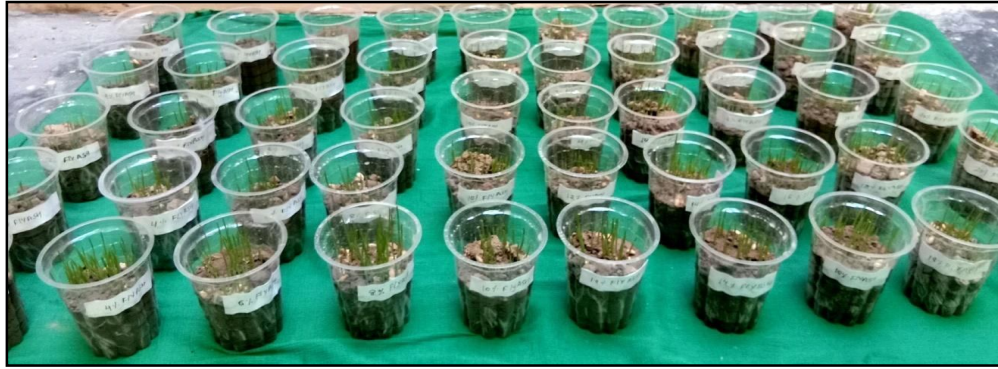
(c): After 5 Days of sowing wheat in different concentrations of fly ash (0%, 4%, 6%, 8%, 10%, 12%, 14%, 16%, 18%, 20%)
