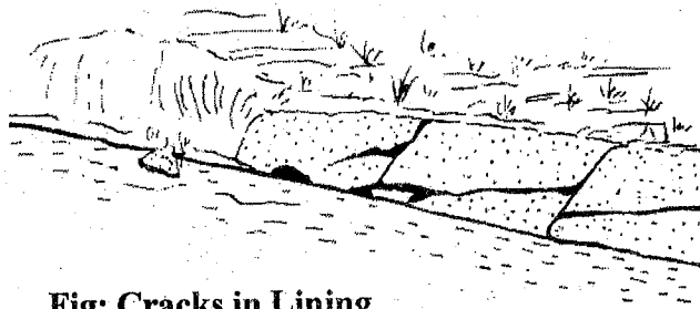
Fig: Cracks in Lining
