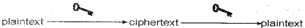
B) Public key (asymmetric) cryptography. PKC uses two keys, one for encryption and the other for decryption.
