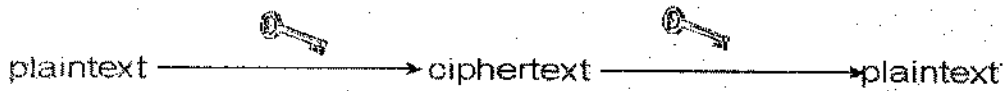
A) Secret key (symmetric) cryptography. SKC uses a single key for both encryption and decryption.
