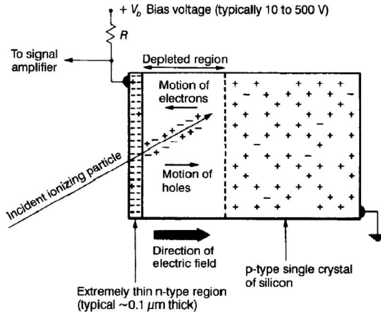
Both surface-barrier and diffused-junction detectors are used for the detection of charged particles. To be able to measure the energy of the incident radiation, the size  $X_0$  of the detector should be at least equal to the range of the incident particle in silicon. The value of  $X_0$ , depends on the resistivity of the material (which in turn, depends on impurity concentration) and on the applied voltage.
