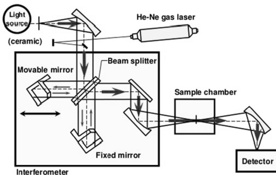
Figure 22.5 FTIR spectrometer
