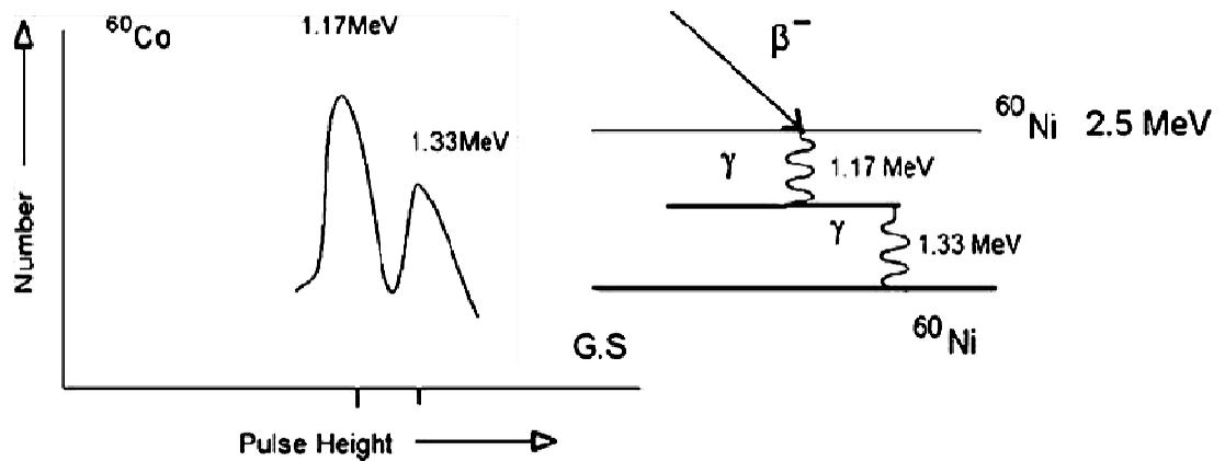
**Figure 10:** (a) Pulse height spectrum of  $\gamma$  -rays of energy 1.17 MeV and 1.33 MeV. The origin of  $\gamma$  -rays is shown in the decay scheme. (b) Decay scheme for  $^{60}\text{Co}$
