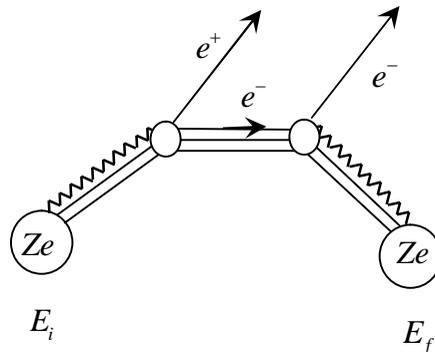
**Figure 11.1:** Pair production in the presence of a heavy nucleus  $Ze$
