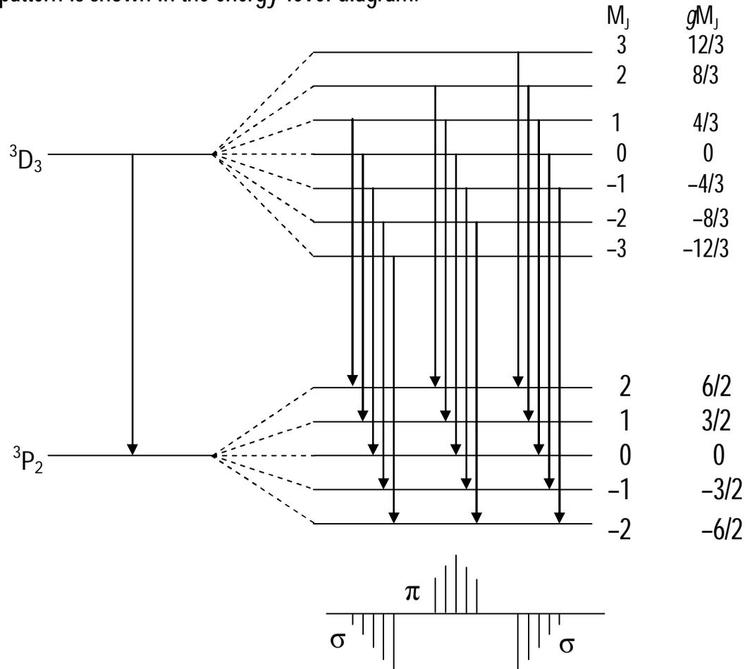
Fig 18. Splitting of  ${}^3D_3 - {}^3P_2$  levels.
