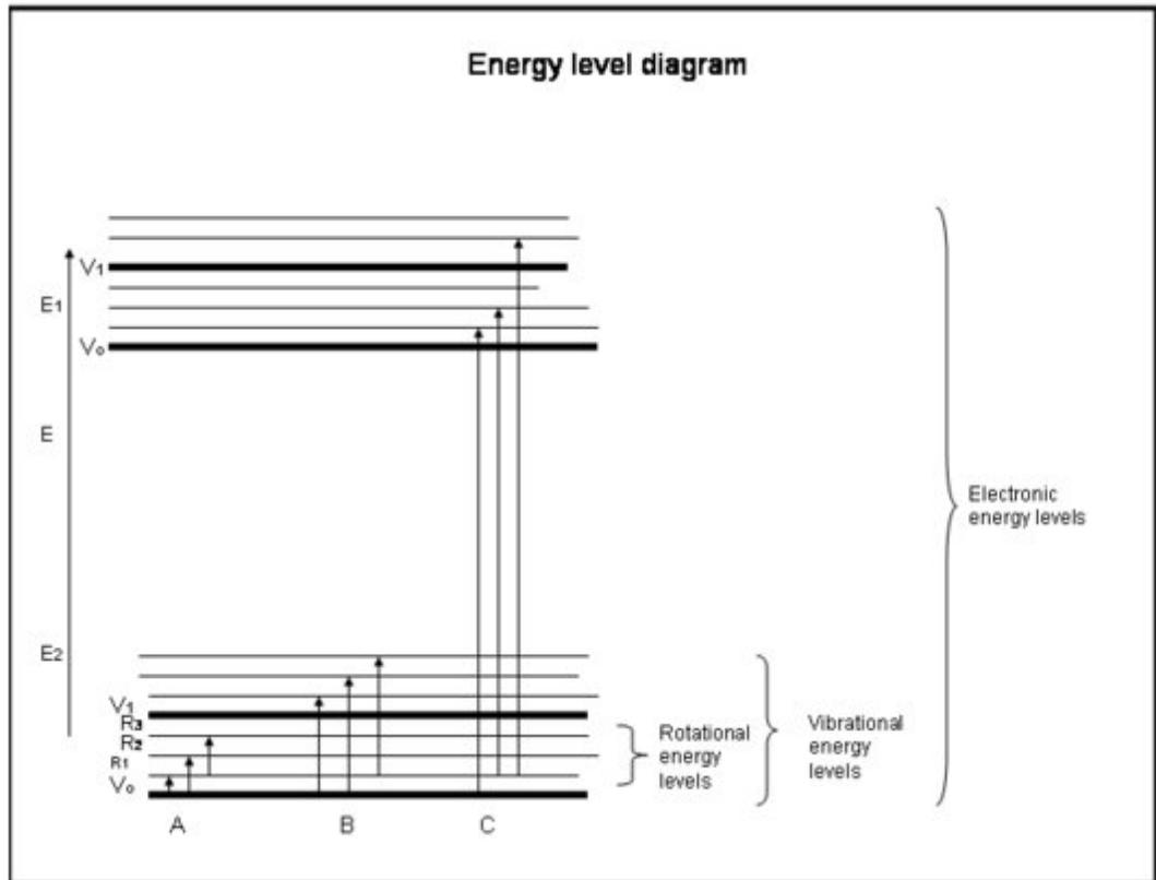
3. Far Infra-red Spectra or Pure rotational Spectra: The vibrational levels are separated from each other by an energy gap of order 0.005 eV. The wavenumber and wavelength corresponding to 0.005 eV is
