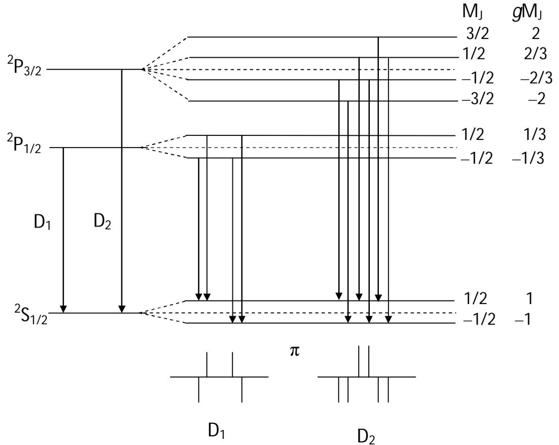
**Fig 8.** Transitions from  $2P_{\frac{1}{2}} \rightarrow 2S_{\frac{1}{2}}$  and  $2P_{\frac{3}{2}} \rightarrow 2S_{\frac{1}{2}}$ .
