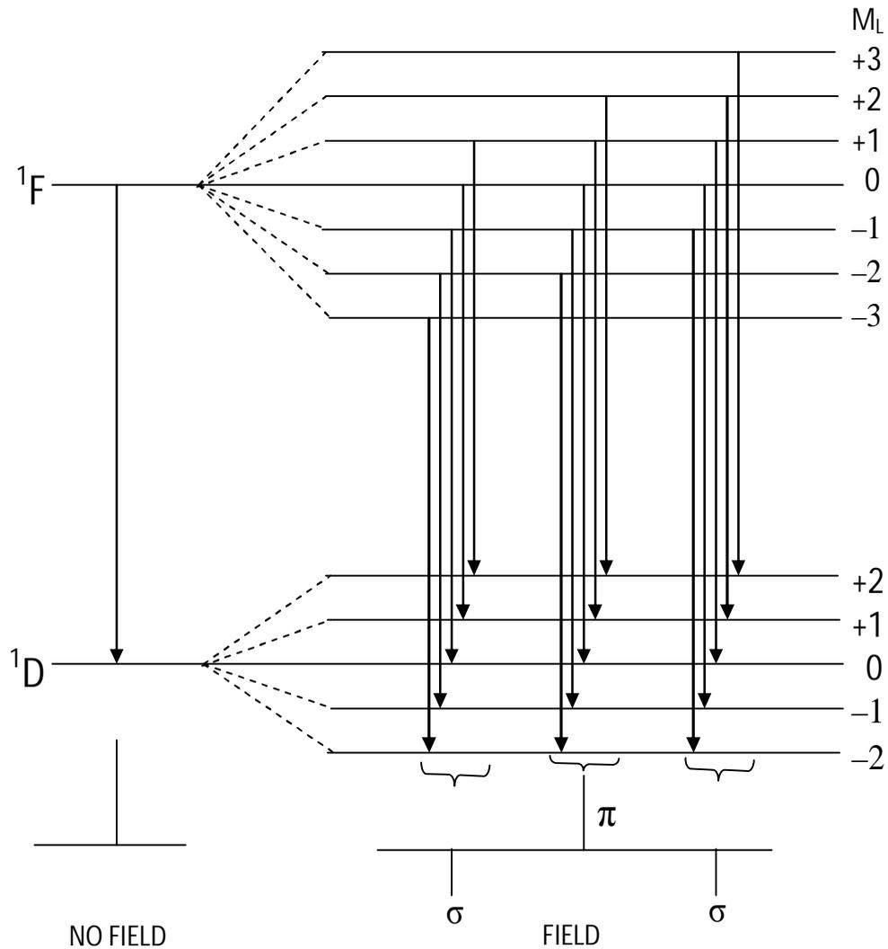
Fig 13. Splitting of  $^1F_3 - ^1D_2$ , single-singlet transition.
