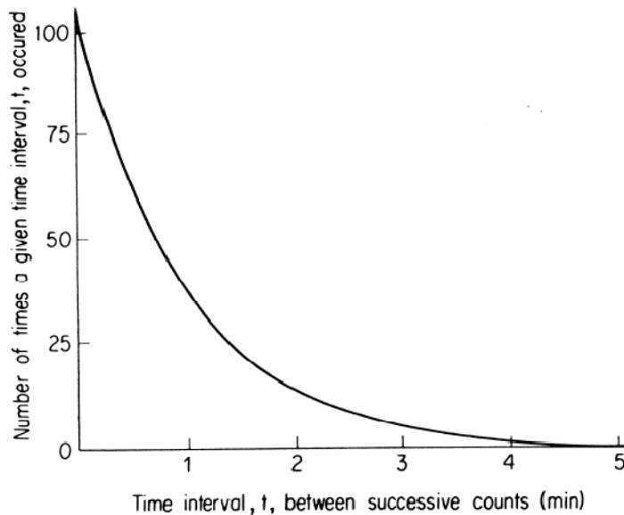
Note the most probable time between events is zero. Random events (counts, natural disasters, etc.) occur in “bunches.” Let us summarize how we describe the statistical uncertainty in measurements of radioactivity. If we measure the activity of a sample (+background) as 64 counts in 1 minute, then we estimate
