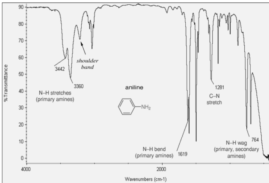
**Figure 22.6. Typical FTIR spectra of Aniline**
