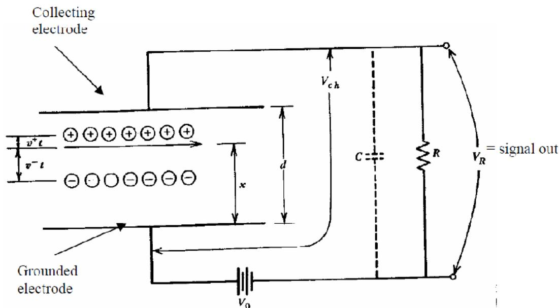
**Figure 4:** *The electronic circuit of ionization chamber*
