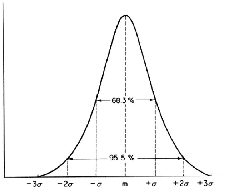
Furthermore 95.5% of all measurements lie within  $\pm 2\sigma$  of the mean and 99.7% lie within  $\pm 3\sigma$  of the mean. The full width at half maximum (FWHM) is  $2.35\sigma$ .
