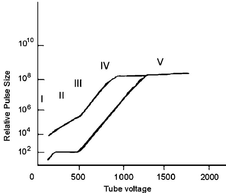
**Figure 2:** Characteristics of a gas filled detector
