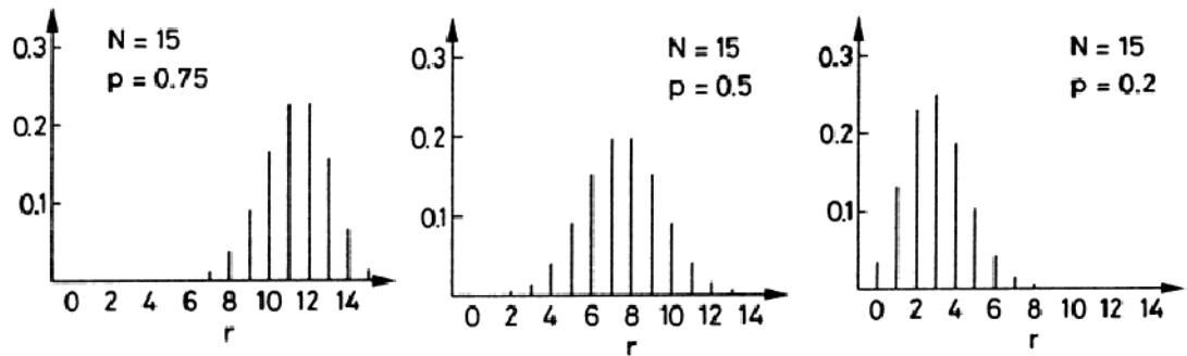
The binomial distribution function is cumbersome and a simplification can be made. If the probability of success  $p$  is small ( $p \ll 1$ ) (the measurement time is very short compared with the half-life), we can approximate the binomial distribution by the Poisson distribution. The Poisson distribution is written as
