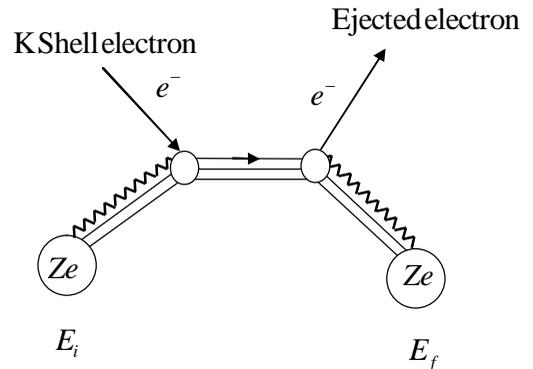
**Figure 11.2 :** Internal conversion of an orbital electron due to electromagnetic interaction with a nucleus.
