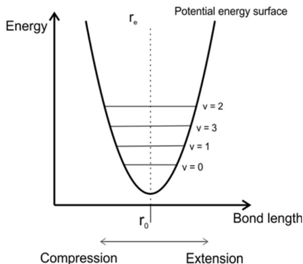
The energy of the vibrational energy levels is quantized. The allowed energies for the diatomic molecule can be determined by solving the Schrodinger's wave equation considering the potential to be harmonic as  $V = \frac{1}{2}kx_0^2$ . The energy of levels of diatomic molecule is given by the following equation
