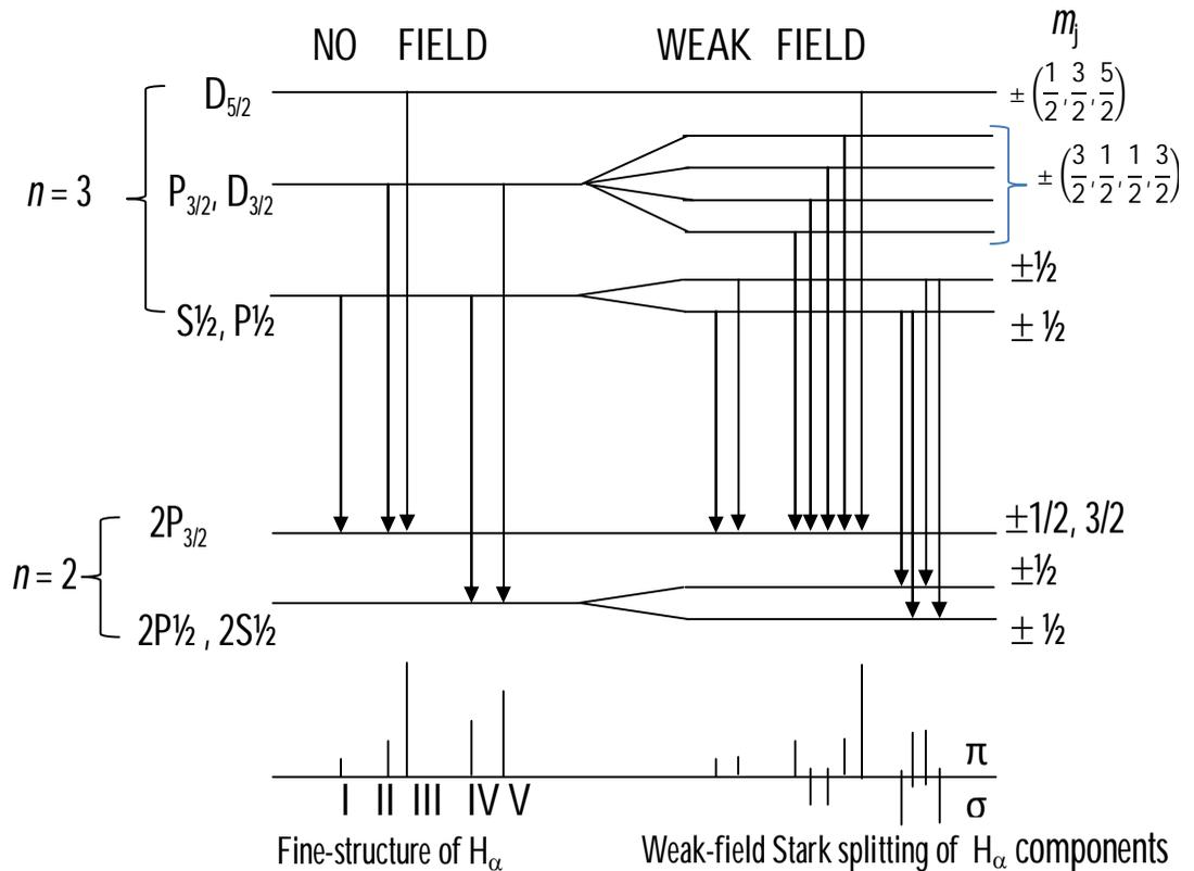
**Fig 20.** Energy levels of H-atom for the transitions  $n = 3$  and  $n = 2$ .
