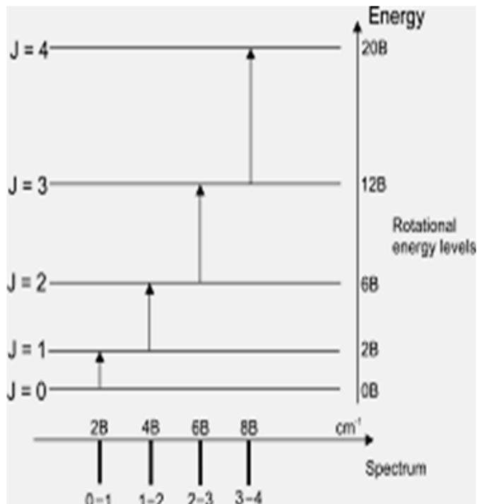
When the transitions take place between an upper level and lower level of rotational levels, then the wave number of absorbed radiation will be
