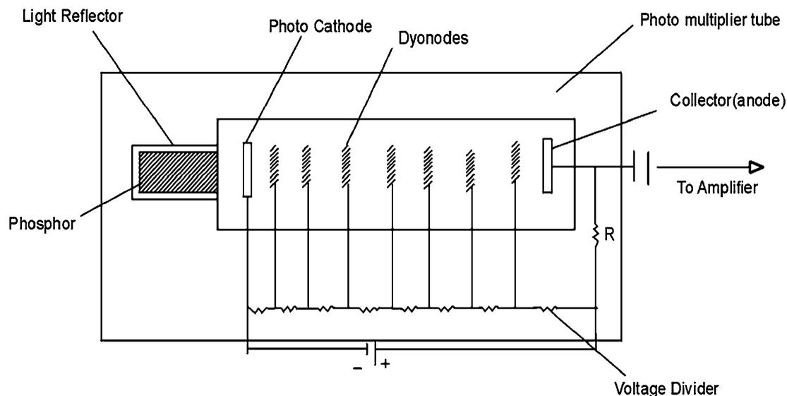
**Figure 6:** Block diagram of a scintillation counter.
