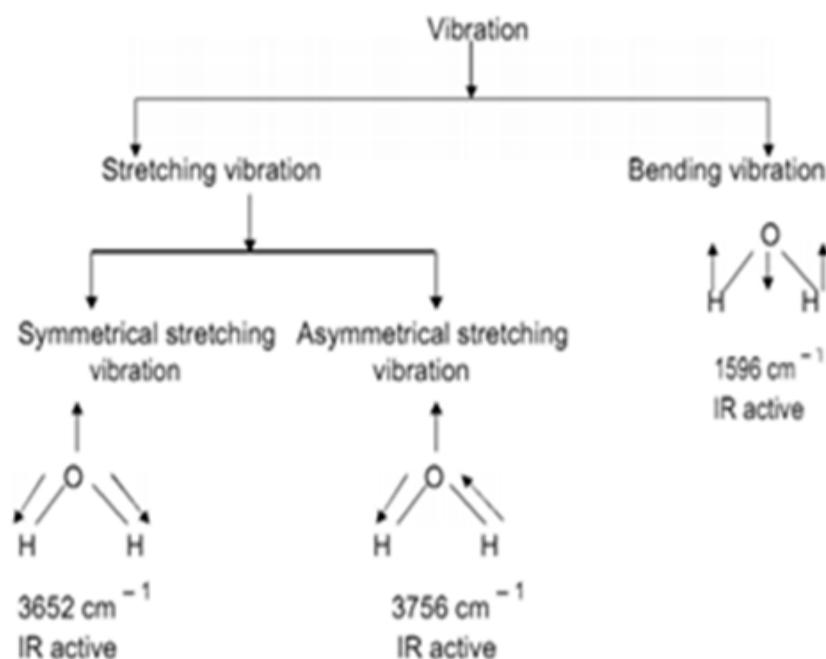
**Figure 22.2 Vibrations of Water Molecule**
