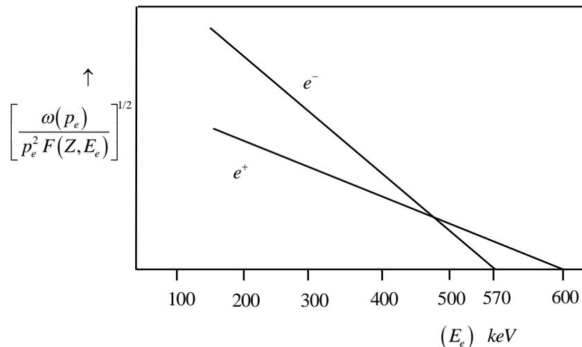
**Figure 10.4 : The Fermi Kurie plot of  $^{64}\text{Cu}$  beta spectra .End points are  $571\text{keV}(e^-)$  and  $657\text{keV}(e^+)$  [Owen & Cook (1949)]**
