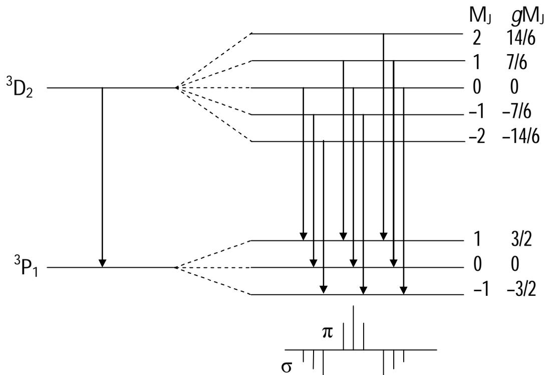
**Fig 17.** Triplet-triplet transition  ${}^3P_1 - {}^3D_2$
