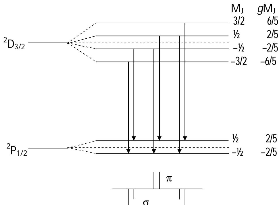
**Fig 14.** Zeeman shifts for the given terms  $2P_{\frac{1}{2}}$  and  $2D_{\frac{3}{2}}$ , doublet-doublet transition
