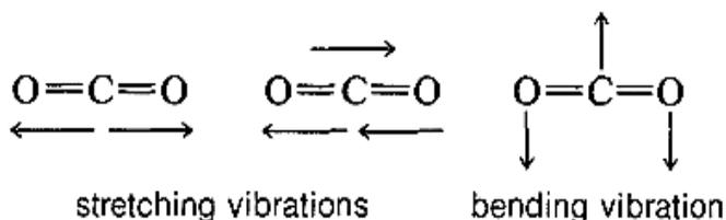
**Figure 22.3 Vibrations of Carbon Dioxide Molecule**
