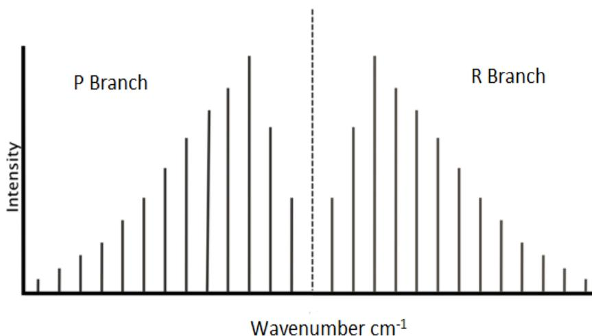
**Figure : Ideal Vibrational-Rotational Spectra**
