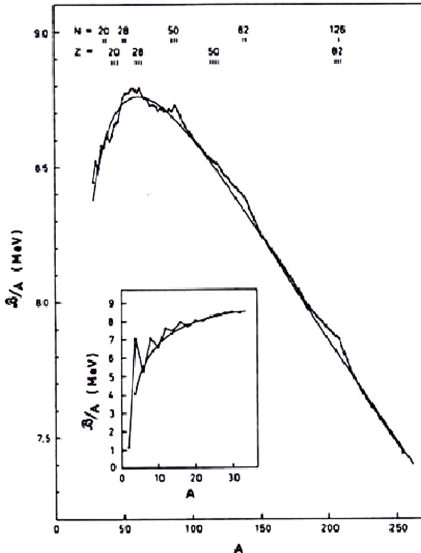
The binding energy curve suggests that nucleons only interact with their nearest neighbours. The range of the force must be less than the size of a mass-10 nucleus, which is around  $1.2 \times 10^{-13} = 2.6$  fm. This property is described as saturation of the nuclear force.
