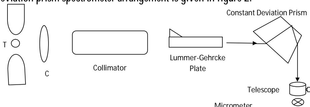
**Fig 2. Schematic diagram of constant-deviation prism spectrometer arrangement.**
