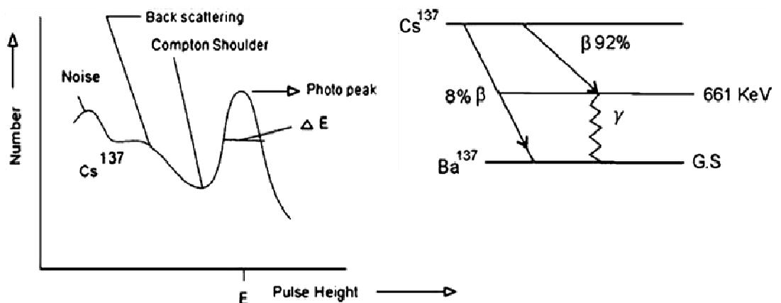
**Figure 9:** (a) Pulse height spectrum of  $\gamma$ -rays from Cs-137 of energy 661 keV. (b) Decay scheme for  $Cs^{137}$
