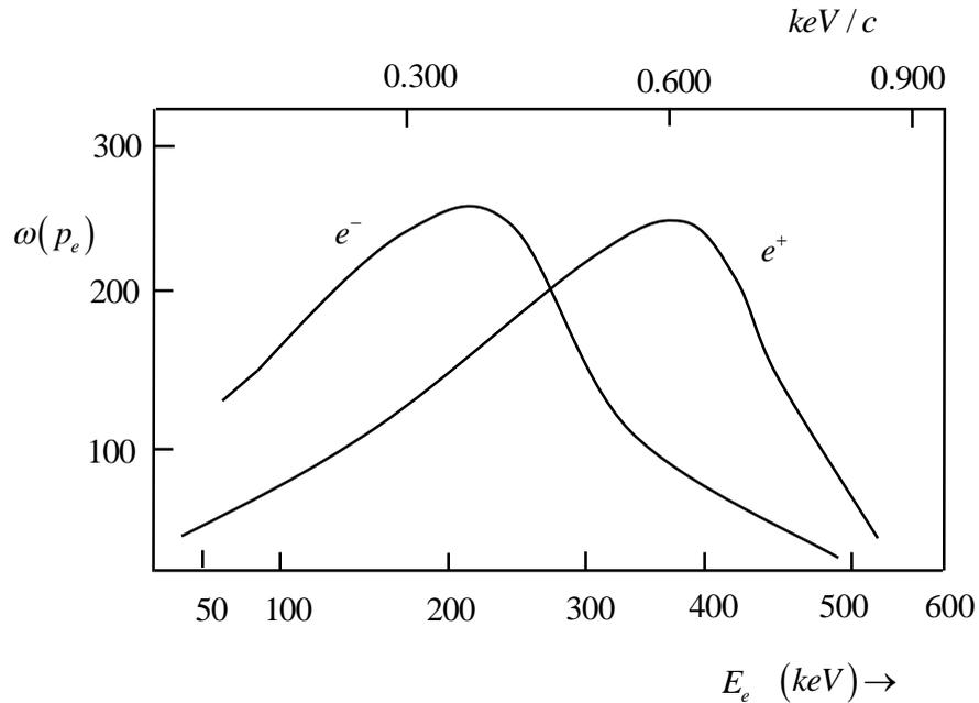
**Fig10.3 : Momentum spectra for  $^{64}\text{Cu}$  electrons and positrons [Wu & Albert (1949)]**
