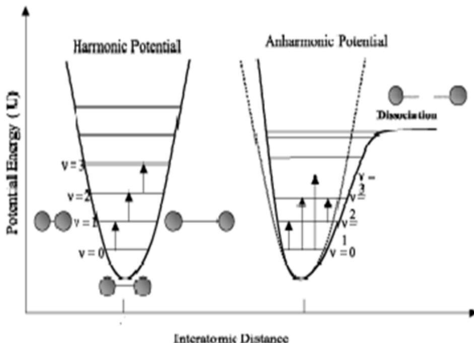
The allowed vibrational levels are given by following equation
