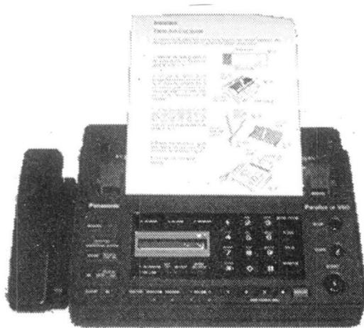
**A Fax machine uses a thermal printer**
